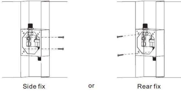
2. Attach face plate to control box.
