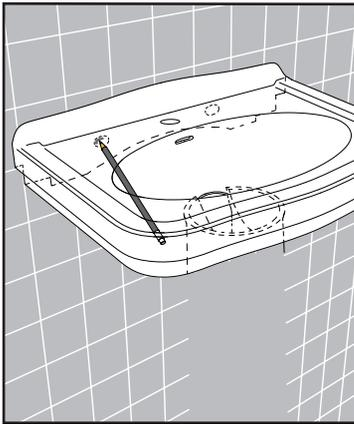
**2** Drill holes in wall for fixings.
