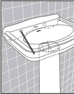
**2** Drill holes in wall for fixings.
