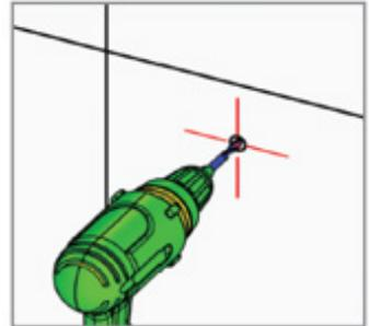
**3** Install fixings and hang basin on wall using level.
