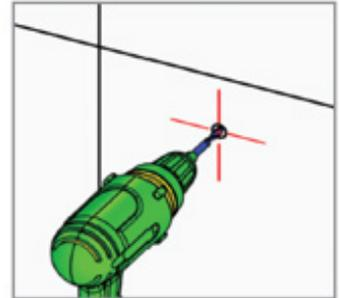
**3** Install fixings into wall, slide basin and pedestal together onto bolts and tighten nuts while using level.
